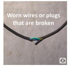
Live cables may be visible in wires or plugs with cracked or frayed outer wrappings resulting in the risk of shock.
