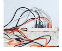
Daisy chaining is when you connect multiple power strips or extension cords together. This can overload outlets and cause fires, damage equipment, or lead to electric shocks.
