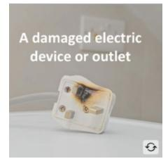
Devices or outlets that have cracked or broken outer covers can expose live wires and electric components.
